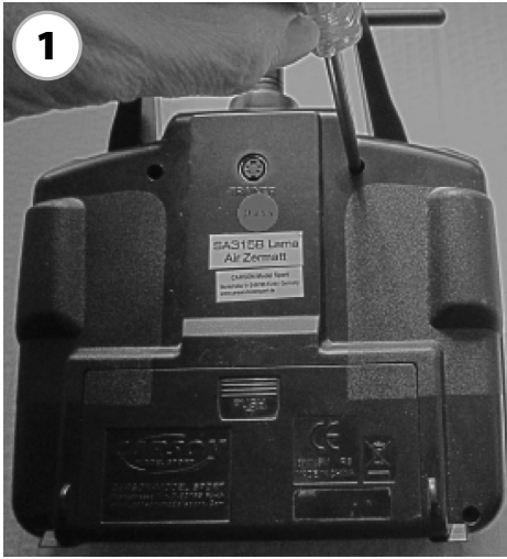
1. Loosen all 4 screws on the back of the transmitter.
